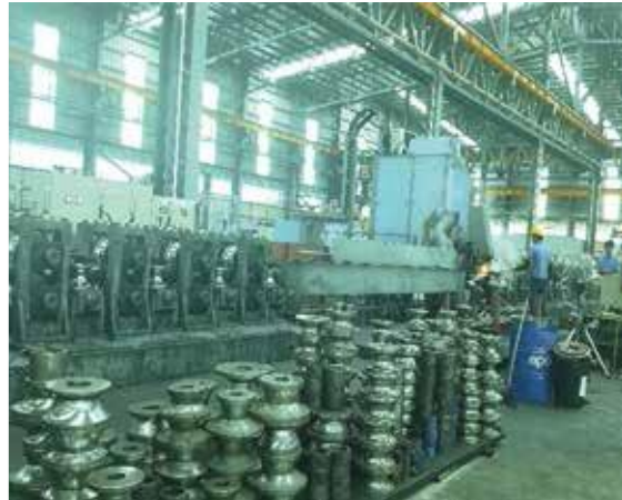
Forming ,Welding, Sizing.
