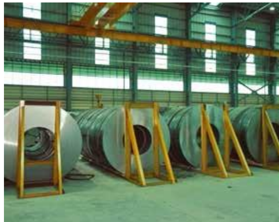
Slit Coil at H-Beam Line
